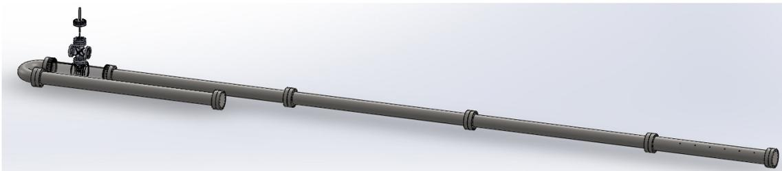
Figure 2.16: Brown Shock Tube, single-pulse constant-area driver solid model
