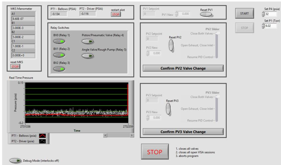
FIGURE 1. Software control panel
